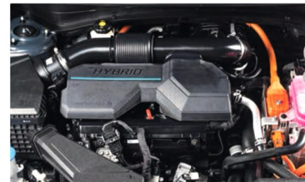
SmartStream G1.6T-GDI HEV Engine Maximum Power: 177 hp Maximum Torque: 265 Nm Motor Maximum Power: 59 hp Maximum Torque: 265 Nm Combined Maximum Power: 227 hp Maximum Torque: 350 Nm Transmission Speed: 6AT
