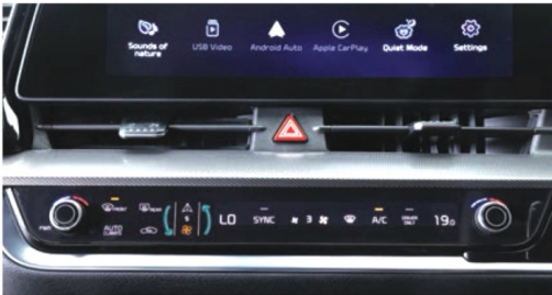
Infotainment/Climate Switchable Controller Infotainment and climate functions share the same LCD softkey keyboard. This improves the intuitiveness and luxury of the cockpit design. Press the fan icon button to transform the controls on the right to climate. Press the arrow icon button to switch them to infotainment.
