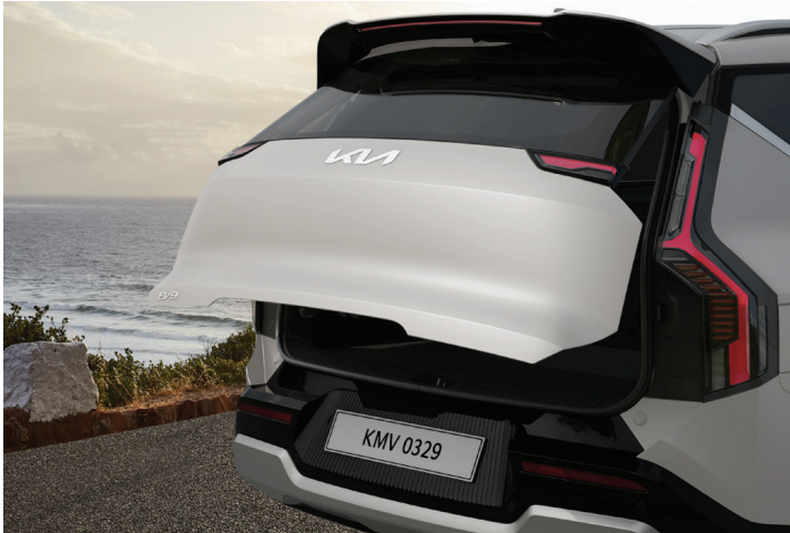
Smart Power Tailgate Simply stand behind the vehicle for three seconds with the smart key in your possession, and the tailgate will open automatically. You can even set the opening height to fit your preferences.
