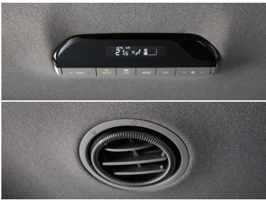
Rear Ventilation System
