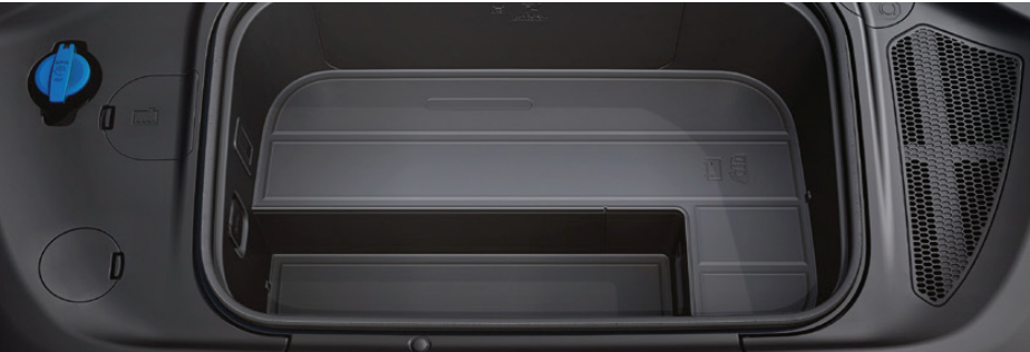
Front Trunk Large-capacity frunk for parcel storage inside the front PE room, with a capacity of 52 liters (max. payload 20 kg)
